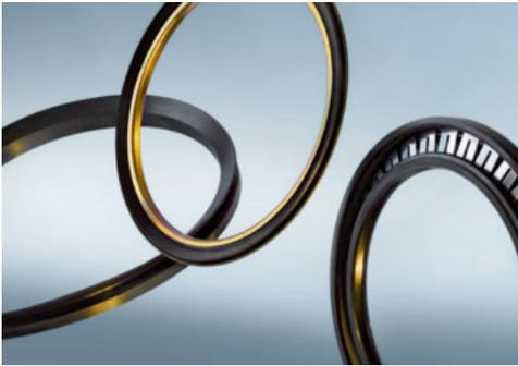
Axial shaft seals are used to seal rotating shafts. The low-friction and wear-resistant seals work axially and are usually mounted securely on the shaft, i.e. the seals rotate with the shaft.
